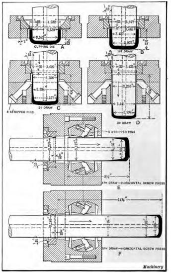
Fig. 25. Dies Used for Drawing 3-inch Brass Shrapnel Cases
